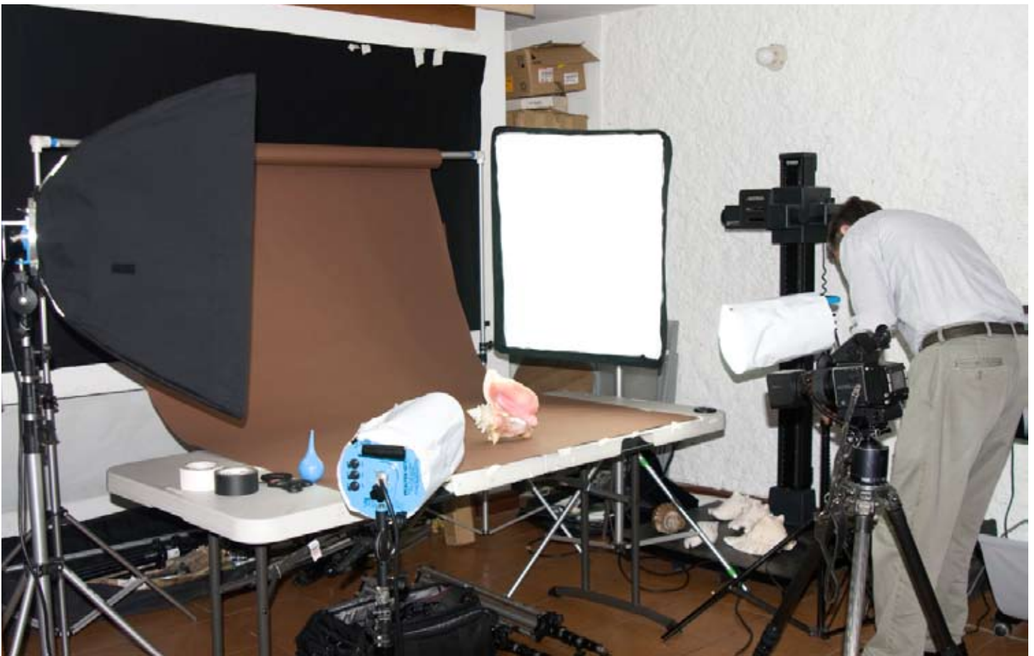
Figure # 5. Our DIY background paper holder (light stands and metal crossbar)
